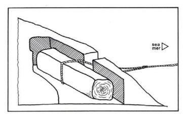
If the boom is anchored to a shoreline, a certain length of boom has to lie on the ground. The shore formation on the site selected for shoreline mooring has to be smooth (sand, gravel) as otherwise the boom damage will result during deployment on rough surfaces (boulders, rocks). The situation may be improved by using bags filled with sand as an "artificial" surface for boom deployment.
