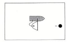
Single vessel system: boom and recovery device deployed from one vessel, generally with the help of a jib.
