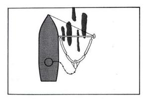
Figure 12 Possibility to combine a boom and a separate skimmer; assembly deployed from a single vessel
