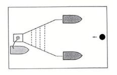
V - configuration: boom and recovery unit towed by two vessels - oil transferred to the third vessel.
