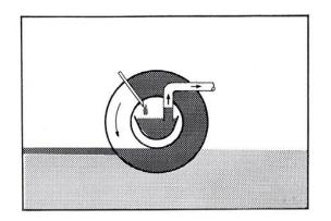
c) <u>Oleophilic belt skimmers</u>: oil adheres to the partly submerged belt made out of an oleophilic material and is carried by the belt movement to the upper part of it, where it is removed either by a scraper (wiper blade) or a squeeze roller.
