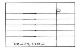
It was discovered that if the current velocity at right angles to a boom's section exceeds a certain value, oil starts escaping underneath the boom. For most of the booms this "critical velocity" is between 0.58 and 0.70 knots (0.30 and 0.36 m/s).
