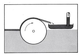
b) **Disc skimmers**: a large family of disc skimmers includes different devices consisting of a variable number of rotating discs made of an oleophilic material. Similarly to drum skimmers, oil which sticks to disc surfaces is wiped by scrapers which direct it into a well (sump, container) from where it is successively pumped out.
