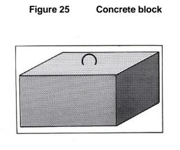
The weight of a concrete block should be at least three times more than the expected load.
