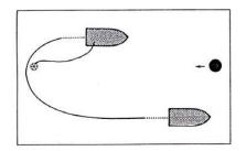
${\sf J}$  - configuration: boom towed by two vessels and recovery unit deployed from one of them.
