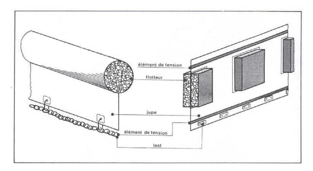
**Flotation element** (float) provides for the buoyancy of the whole system (boom), but often functions as an additional freeboard to reduce splash-over. It can be filled either with some solid material (expanded plastic foams e.g. polyethylene, polyurethane, polystyrene or natural flotation materials e.g. cork, wood, etc ...) or with air.
