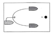
U - configuration: boom towed by two vessels and recovery unit deployed from a third one.
